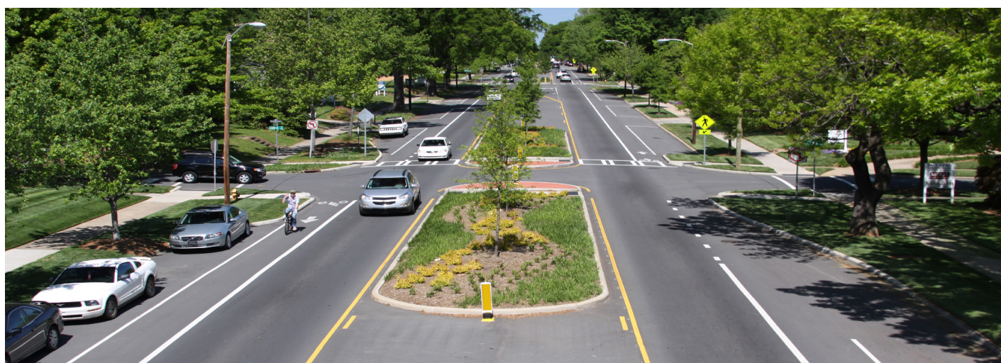
A road diet on East Boulevard in Charlotte, N.C., reduced travel speeds, bicycle and pedestrian injury rates and the number of rear-end and left-turn collisions. (Photo courtesy city of Charlotte)
