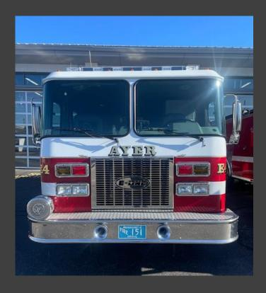
Engine – 4 1993 E-One Protector 1250 GPM pump 750 Gallons of water 30 Gallons of foam
