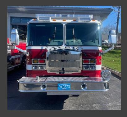
Engine – 2 2020 E-One EMAX 1500 GPM pump 750 Gallons of water 30 Gallons of foam
