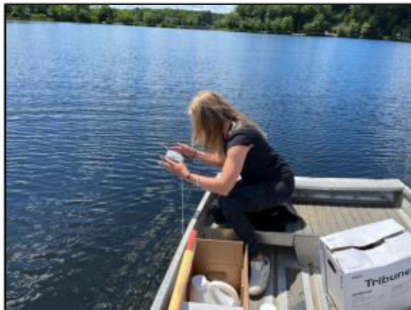
Figure 2 Collection of Secchi disk data at Sandy Pond
