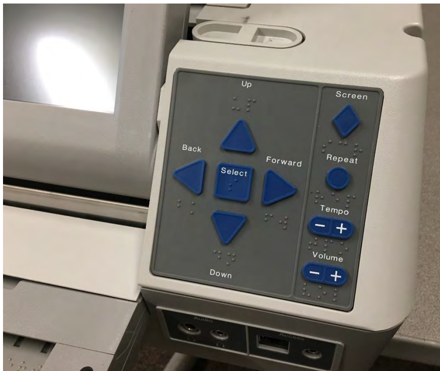
(Town of Ayer – Close-up control panel with Braille of the municipal AutoMark Voting Machine)
